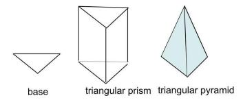
Volume of a Prism: V = Bh, where B represents the area of the base and h represents the height of the prism
